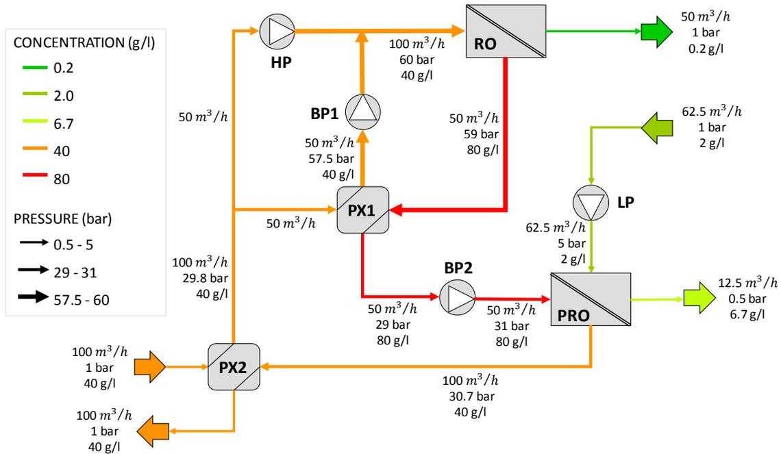
Fig. 1. Schematic diagram of the first SWRO+PRO arrangement proposed in the patent analysed.
