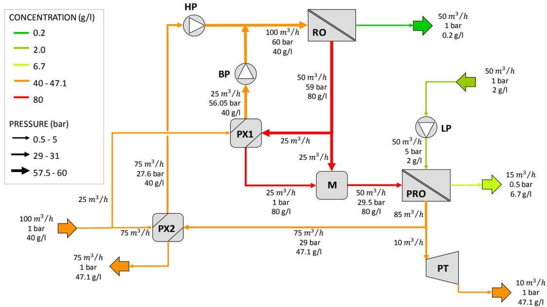
Fig. 3. Schematic diagram of the third SWRO+PRO arrangement proposed in the patent.
