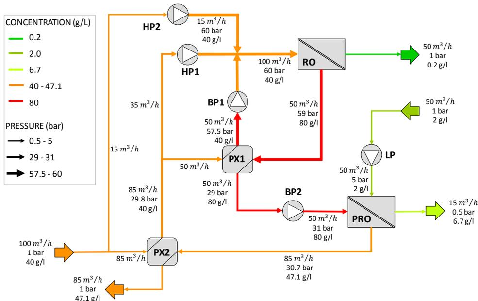
Fig. 2. Schematic diagram of the second SWRO+PRO arrangement proposed in the patent.
