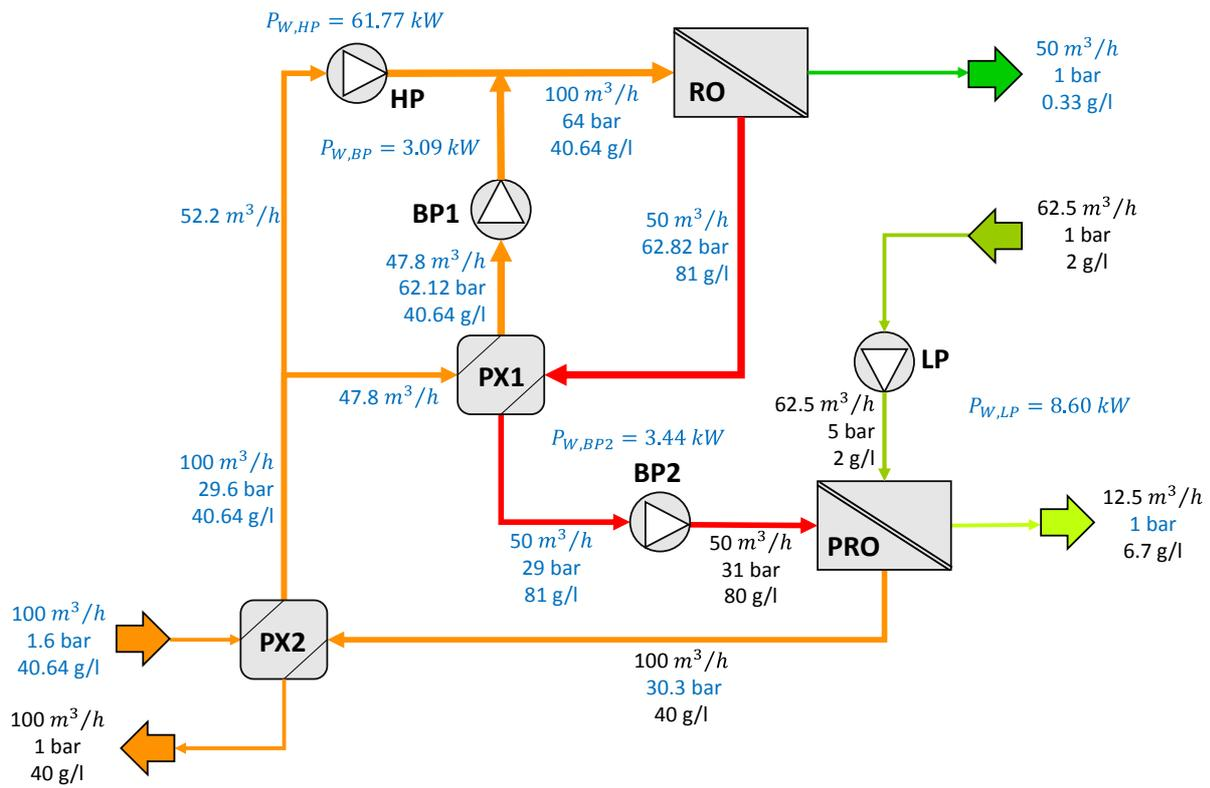
Fig. 6. Results for the first configuration of the patent. Black values are taken directly from the patent and blue values are calculated.
